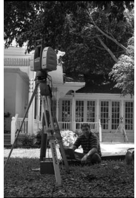
SCAN DATA WAS COLLECTED FROM 26 EXTERIOR LOCATIONS AND THEN COMBINED INTO A SINGLE POINT CLOUD THAT IS BEING USED TO CREATE A 3D MODEL.
