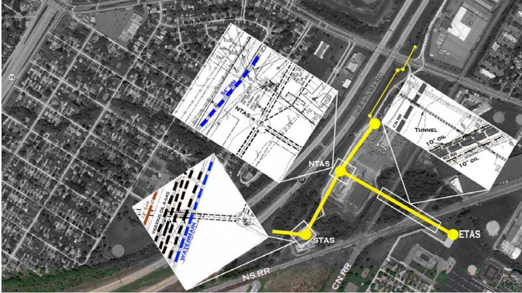
Figure 2. Critical utility crossings
