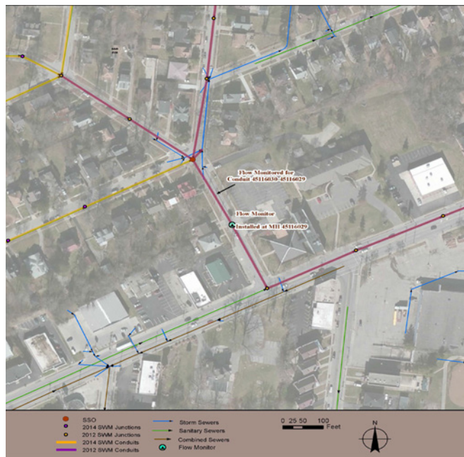
Figure 8 Location of SSO 228 flow monitor.
