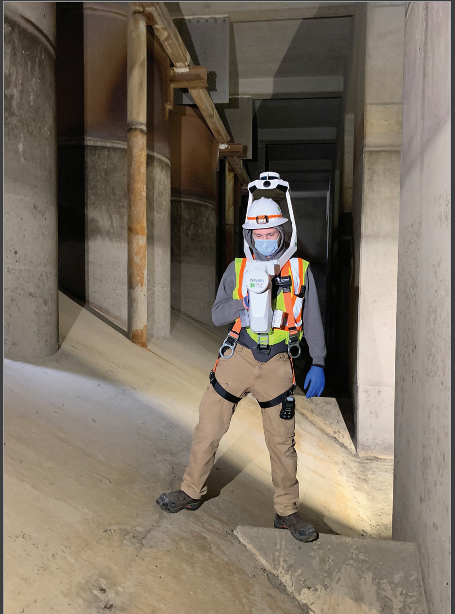
Reality capture during inspection improved safety and increased data retrieval efficiency in areas with complex geometry and confined space constraints. The information helped facilitate planning and desktop evaluation of existing conditions. Photo courtesy of Wade Trim
