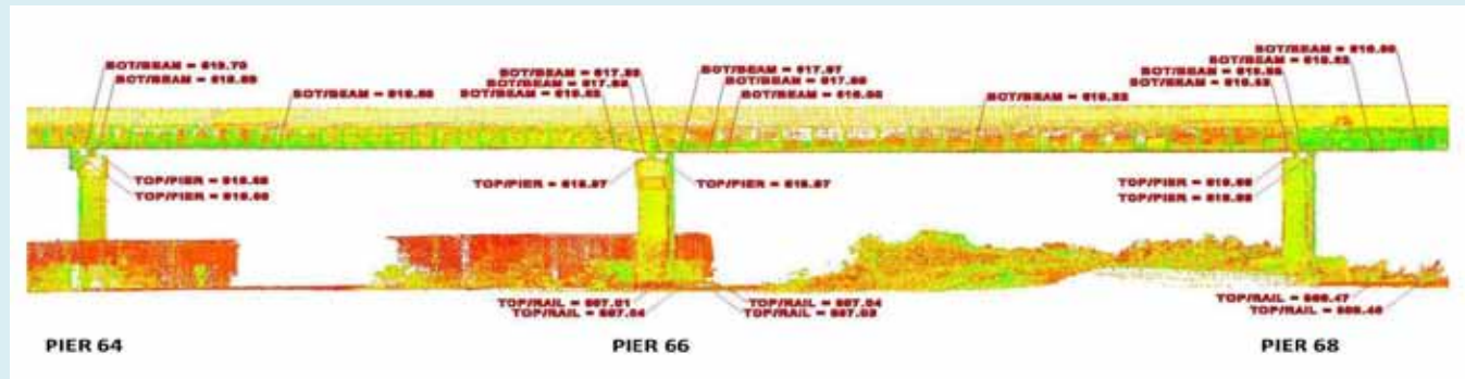
STLS scanning under the bridges allowed all underclearance and offset dimensioning to be shown on digital scans with near photographic quality.
