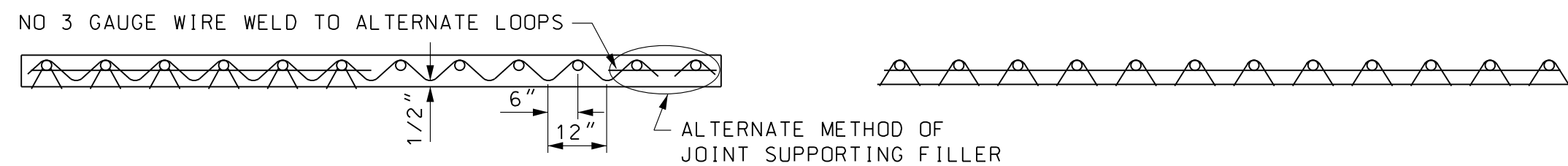
SECTION A-A EXPANSION BASKET ASSEMBLY SIDE ELEVATION CONTRACTION BASKET ASSEMBLY
